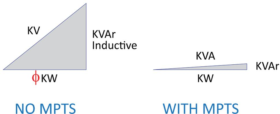
The MPTS does not change the Power Factor directly. It continuously adjusts the impedance matching on the power line, thereby reducing reactive power consumption. MPTS also reduces Total Harmonic Distortion (THD) by reducing total current (Amps) consumption. MPTS thereby minimizes magnetic core material nonlinearities in motors and transformers, which are a major source of harmonic distortion.
